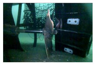
Figure 77: Lady Gertrude on the ocean floor. The propeller shaft has backed out of the stern tube and the shaft locking nut is jammed against the balanced rudder. PHOTO BY DEPTH CHARGE MARINE
