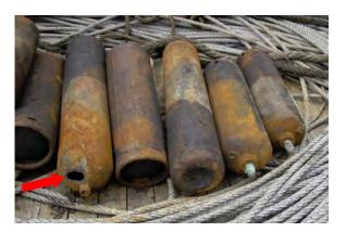
Figure 44: Oxygen and acetylene bottles on deck post-fire. Arrow shows a hole at the melted pressurerelief fusible plug location on one of the bottles. PHOTO BY COAST GUARD
