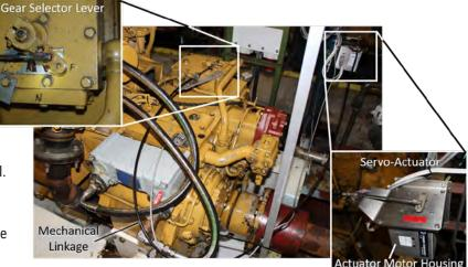
Figure 3: Port ZF marine transmission with close-up of the gear selector lever for the mechanical control unit in the forward position as found immediately after the accident. Also shown is a close-up of the Twin Disc control system servo-actuator. PHOTOS BY COAST GUARD & NTSB
