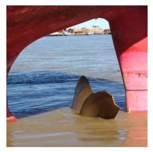
Figure 18: Nordbay's damaged propeller. PHOTO BY DNV-GL
