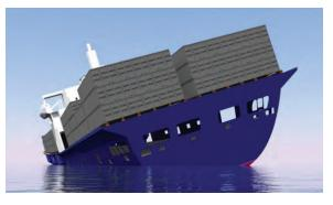
Figure 67: El Faro computer rendering in static surface water showing list to port of 18° with departure trim 5.8 feet by the stern due to flooding of hold 3, estimated at 20% and windheel. ILLUSTRATION: USCG MARINE SAFETY CENTER
