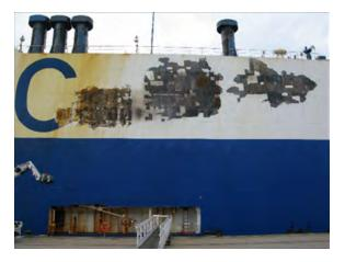
Figure 49: Exterior damage to *Courage* starboard side in the vicinity of the fire. PHOTO BY COAST GUARD
