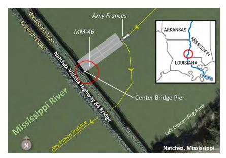
Figure 6: Satellite image of the accident site overlaid with a graphical depiction of *Amy Frances* tow and automatic identification system (AIS) track data. BACKGROUND BY GOOGLE EARTH PRO
