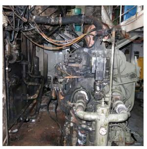
Figure 59: Damaged starboard engine aboard *The Admiral* after the fire.
