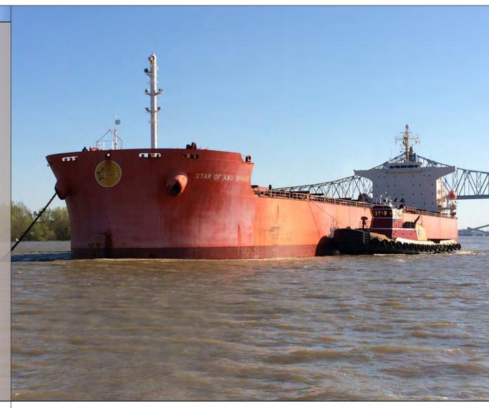
Figure 21: Star of Abu Dhabi after the accident, with missing port anchor. PHOTO BY COAST GUARD
