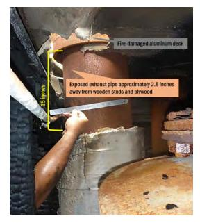
Figure 53: An investigator measures the distance between the wooden studs and the exhaust pipe of *Raffaello's* starboard generator, on which a 15-inch section of insulation is missing at the top. PHOTO BY COAST GUARD
