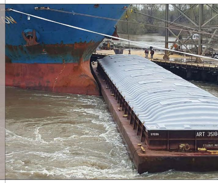
Figure 38: Barge ART 35184 wedged under the dock after the Crimson Gem tow collided with the bulk carrier Yangtze Ambition. PHOTO BY COAST GUARD
