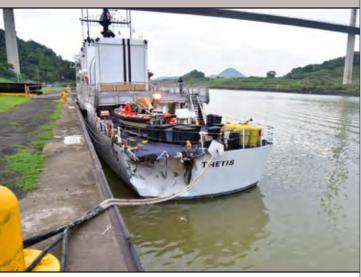
**O** n June 2, 2016, about 0111 local time, the dump scow barge 123 being pushed by the towing vessel *Matachin* collided with the US Coast Guard cutter *Thetis* in Las Cascadas Reach, Panama Canal. Although the *Matachin* and its tow were undamaged, the *Thetis* sustained an estimated \$1.2 million in damage to the hull and deck plate aft, as well as to various systems in the steering gear room. No one was injured, nor was any pollution reported.
